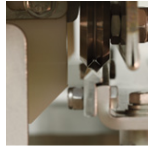
V-groove roller bearing, moveable table.
