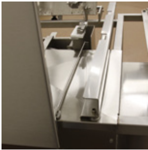
Water Spray pre-attached blade cleaning system.
