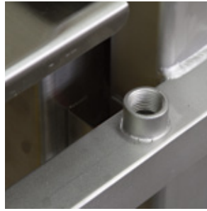
Frame clean-out flushing port.
